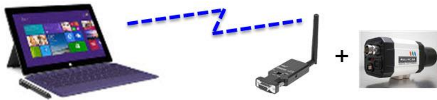
SECTION A: Laptop Bluetooth connection to SIIG Bluetooth module
